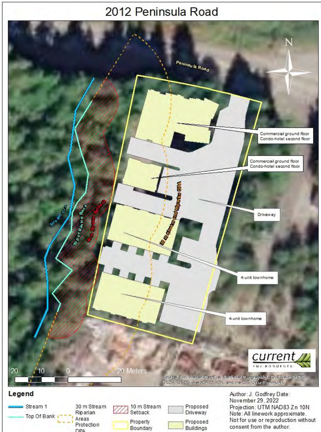
Figure 3: Site Plan of proposed development on the subject property (Development extending to neighboring property not shown) in relation to Stream 1 and associated SPEA.
